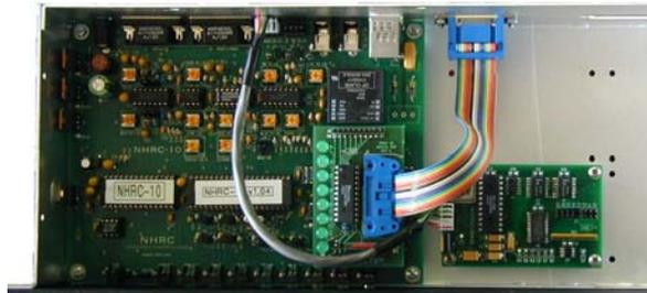
NHRC-10 shown mounted in the NHRC-10/CAB with optional NHRC-10/DOUT and NHRC-DAD boards installed
